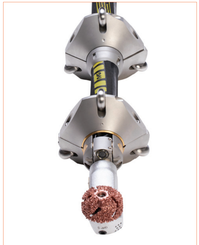
Spotfacing Indicator on Centering Rings: Each centering ring has a spotfacing to indicate which side should face the grinder. Make sure this is correctly aligned during installation.
