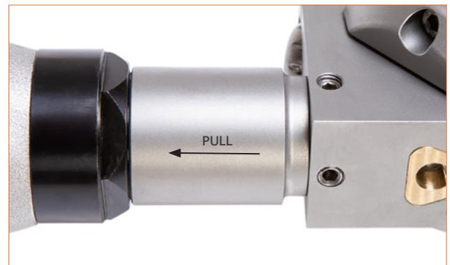
1. Loosen the three screws with the hex key
