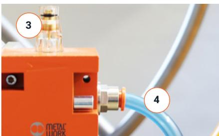
**If the system has to be laid down during transport, un screw the oil-lubricator glass to prevent oil from entering the cleaner tank.**
