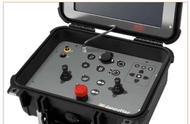
Open the lid of the control unit and loosen the emergency stop button. Turn on the camera light, if necessary.
