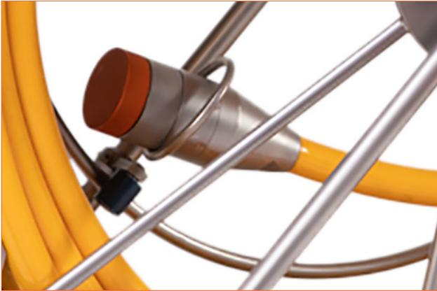
Feed the plug on the yellow hose through the ring on the reel, pull out a short section of hose and lay it on the ground.
