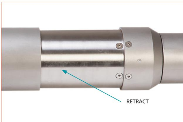
ALWAYS retract the forward/back drive section before moving from one position to another in a pipeline. (7.4: "3")
