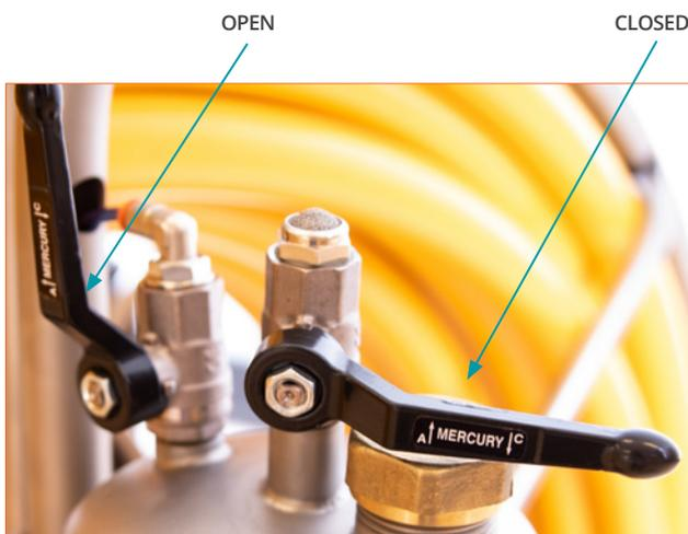
Now open the ball valves supplying air to the tank.
