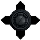
**RIGHT JOYSTICK:** Use the up/down to raise and lower the grinder on the cutter. Use the right/left to rotate the cutter.
