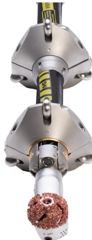
There is a spotfacing on each of the centring rings to indicate which side of the ring should face the grinder.
